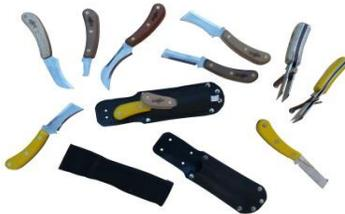
Straight bladed Safety Knives--- Hand made straight bladed grafting knife with safety features for whip and tongue grafting. Yellow high visibility plastic handle. Supplied with leather carry and storage sheath. Available in right and left handed models. Some models have extra guards for safety when doing whip & tongue grafts by hand.
